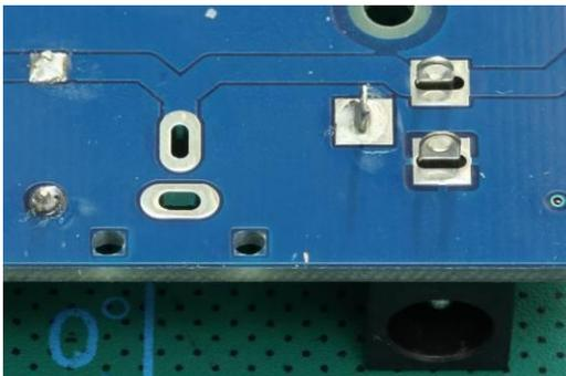
Partially solder one pin and check the socket hasn't moved.
