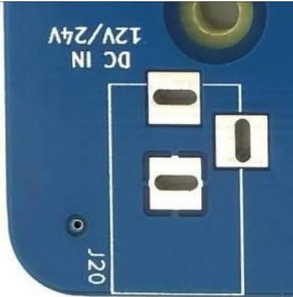
Don't be shy with the solder here. The barrel jack will have stress from plugging in and pulling out the power supply plug so add a bit more solder.
