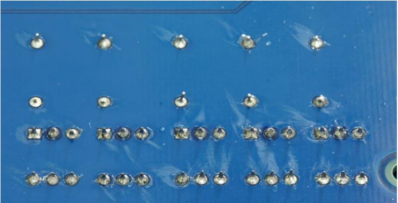
This can be cleaned up using Isopropyl Alcohol, a small brush (old tooth brush is fine), and some elbow grease.
