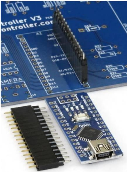
Use the PCB to support the headers with pins inserted.
