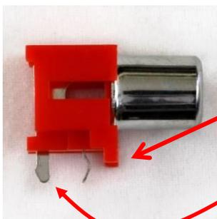
The feet at the front fit in to the holes in the PCB.
