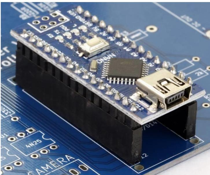
Solder the Arduino pins.
