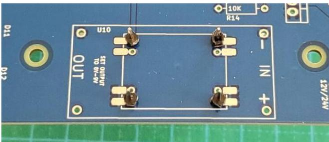
Place the 4 pins in the PCB as shown in the photo.
