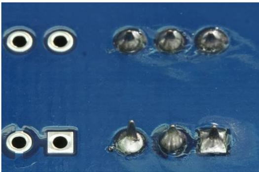
Remember you need to keep the pins separate. If you inadvertently join two pins together, remove the solder and try again.
