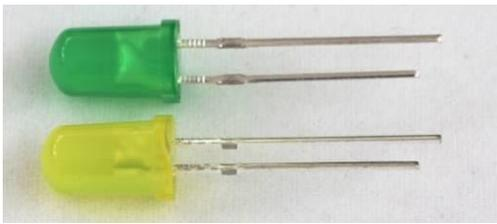
LEDs normally have a long pin and a short pin\*. The long pin goes through the circular hole\*\*. After inserting, separate the pins slightly to stop them falling out while you solder them.
