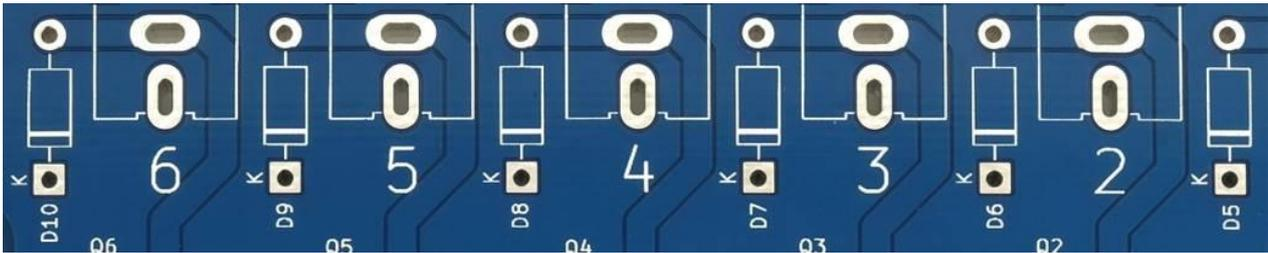
After completing the resistors move on to the diodes. Diodes are electrical one way devices (not really true but close enough) and if you get them the wrong way round the resultant explosion will destroy the planet\*.
