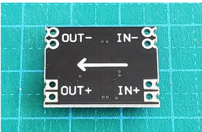
Make sure you have the buck converter in the correct direction
