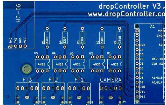
To help make assembly a little easier extra space has been added to the PCB layout. There are some tight spaces though; such as the pins on the Arduino and the IC sockets.
