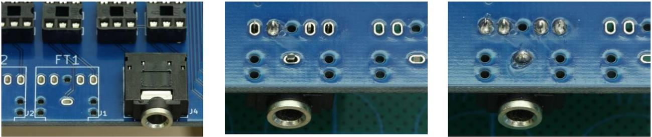
Make sure the socket is flush to the PCB. The pins should be fully through the PCB and the small tabs on the bottom of the sockets should be in the 4 holes.
