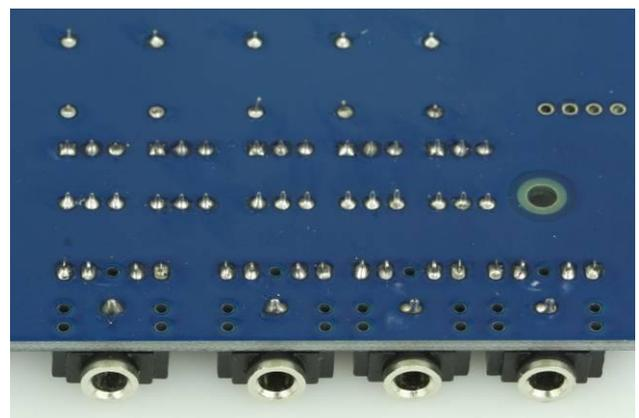
Double check that pins are not joined together.
