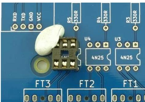
Getting the socket to stay in place when you flip the board over can be finicky. A small blob of Blu-Tack can help.
