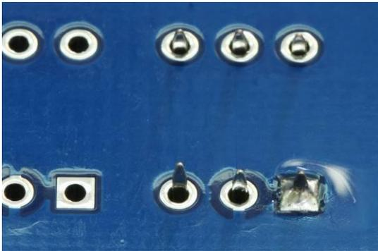
Solder a corner pin first then check the socket hasn't moved before soldering the remaining pins.
