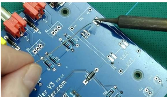
Tin the pads where the converter will go. Just need to add a small amount of solder.
