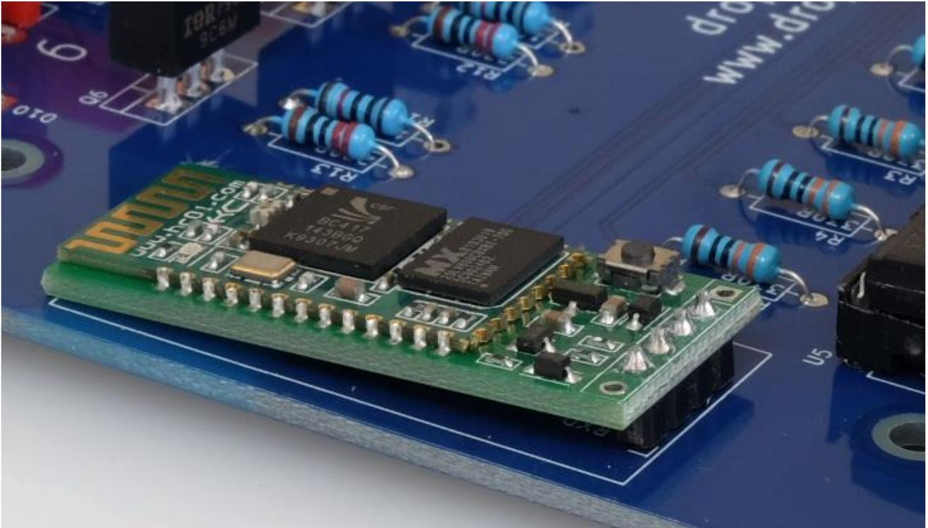
The Bluetooth module is at a slight angle so that the bottom of the board is against the PCB.
