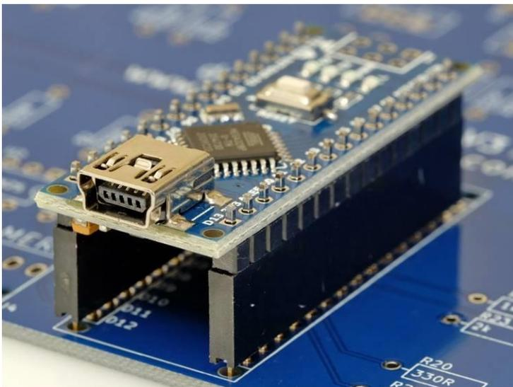
Add the Arduino on top of the pins.
