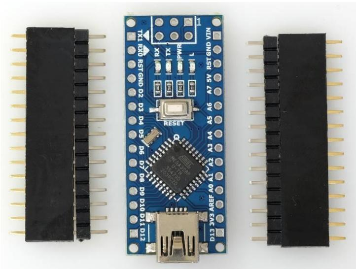
Start by inserting the Arduino pins into the headers
