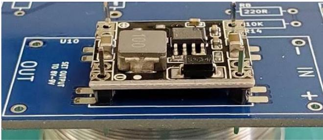
Place the buck converter on the pins
