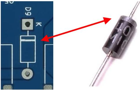
On the diode there is a white (it's actually grey or silver) line at one end, align this with the line on the PCB.
