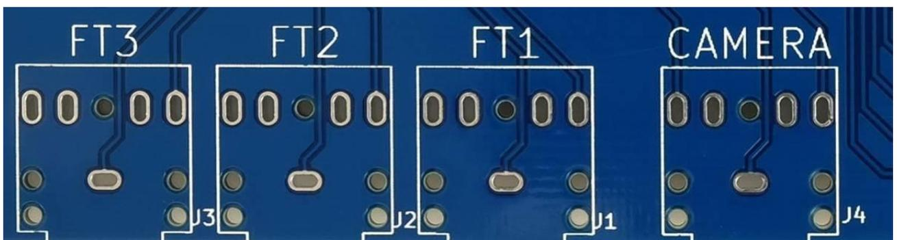
As with the optocoupler sockets, start by soldering one pin, check the position, then solder the other pins.
