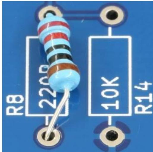
When the pins are bent sharply the resistor will want to sit at one end on top of a hole and will not lie flat.
