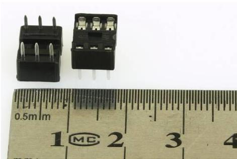
The pins are now starting to get closer together. If you are not that experienced with soldering just take your time and remember to heat the pin as well as the solder. We are not talking white hot here! About half a second contact with the soldering iron should be enough. Solder will flow nicely on a hot pin and recoil in horror from a cold one.
