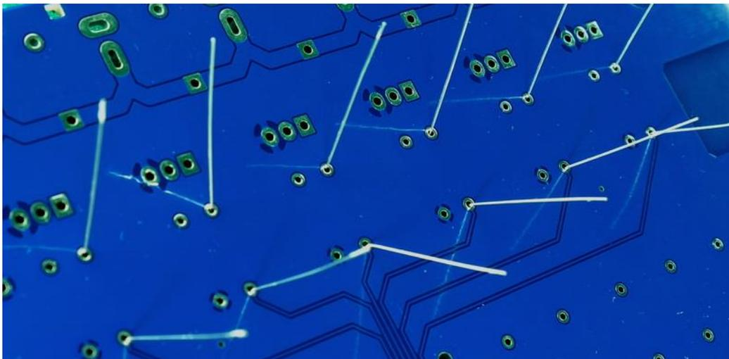
When inserting the resistors, separating the pins slightly helps keep the resistors in place when flipping the board upside-down.
