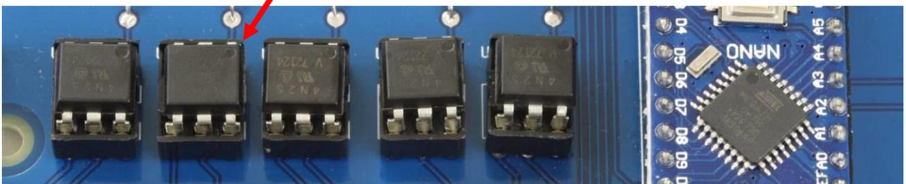
Make sure the pins are securely inserted in to the sockets and not bent.
