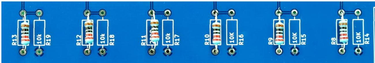
A nice touch is to place all the resistors in the same orientation so the coloured bands line up.
