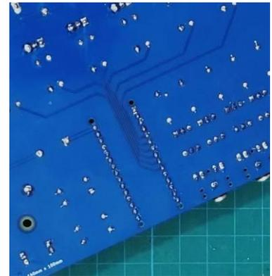
Solder one corner then check that the headers are still in position and are lying flat. Solder the opposite corner and check again.
