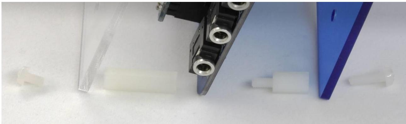
For each corner there is 1 short support, 1 long support and 2 screws. If you have short screws use them at the bottom. All the bits screw in to each other:
