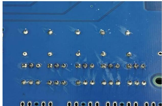
When done check for solder bridges/shorts that join pins together. If you have any shorts, remove the solder and re do. This is important. The camera and flash triggers will not work if pins are connected together.
