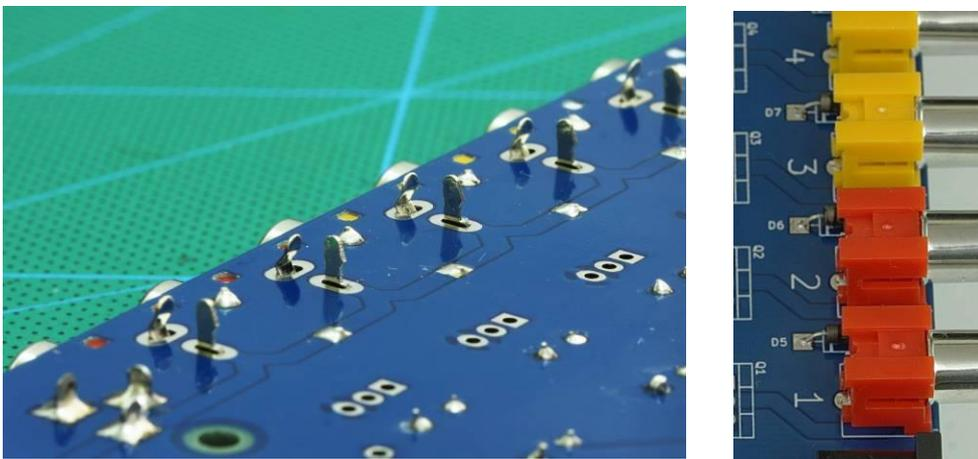
The phono sockets are another high stress part that benefit from a little more solder\*. Warm the pins and pads before adding the solder and let the solder run around the joint. Do not get it that hot that you melt the plastic and set fire to the PCB though.
