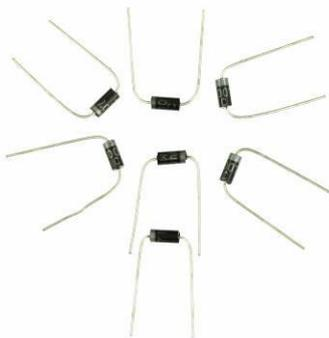
As with the resistors, bend the legs from the end of the leg so you get a nice round corner.
