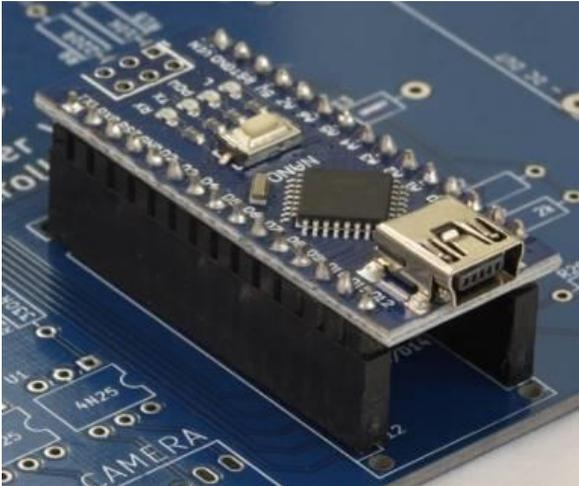
After soldering the Arduino pins, flip the PCB upside down and solder the headers to the PCB
