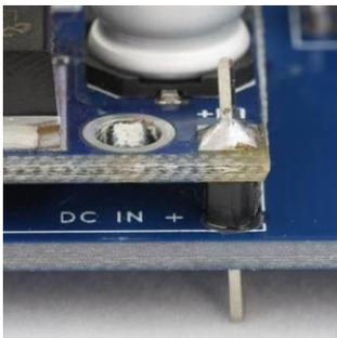
Solder the pins to the buck converter first. Then flip the board over and solder the pins to the PCB.
