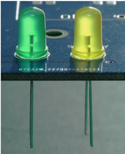
Try to get the LEDs flush to the PCB.
