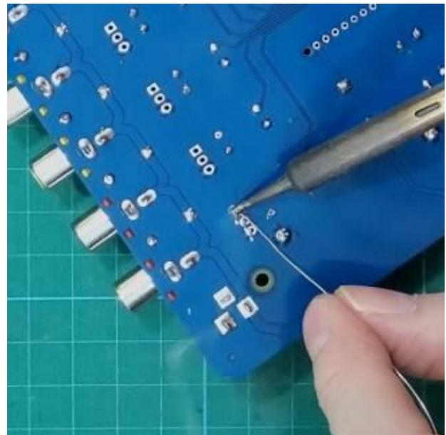
After soldering the first pin, check the position of the mosfet and if it didn't move while soldering do the remaining two pins.
